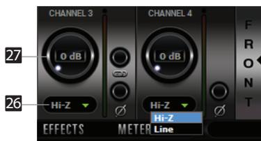
26. Mic and Line (Rear inputs on TRS / XLR combo) modes selectable via dropdown menu (please ensure your selection from the dropdown menu matches the type of signal being inputted)
