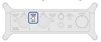
**3.** Press PHANTOM POWER so that they light when connecting condenser mics.
