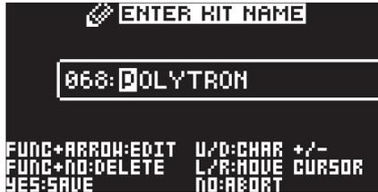
The **[LEFT]** and **[RIGHT]** arrow keys are used to navigate between the letters. Turn the **TRACK LEVEL** knob or press the **[UP]** or **[DOWN]** arrow keys to select the letter. **[FUNC]** + **[NO]** will erase letters.
