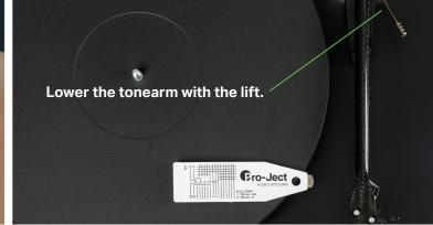
Place the stylus on the gauge. The stylus should read 20.
