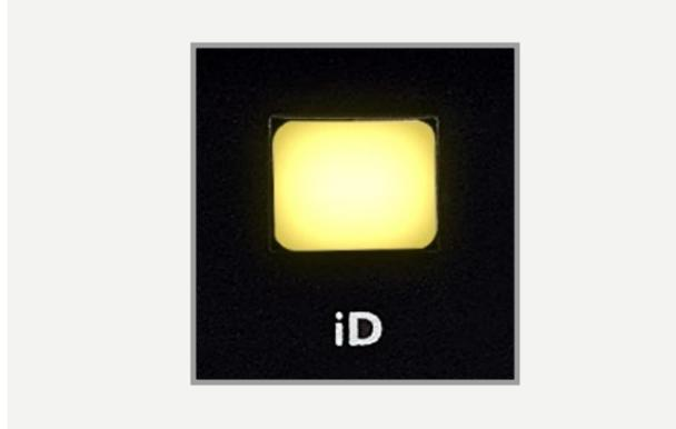
The iD button switches iD44 into **ScrollControl** mode, allowing the encoder to be used as a scrollwheel for the computer. This gives you the ability to control plugin parameters and anything else that is scrollable. This works well for adding automation or setting parameters in a hands-on way.
