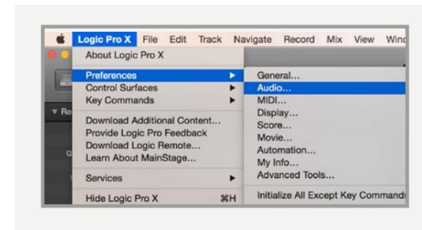
Ensure that iD44 is selected as the active audio device and set the buffer size (to affect system latency). If you are experiencing issues with playback stability and CPU loading, try increasing the buffer size. This appears with "overload" errors and/or pops and clicks and distortion in the audio.
