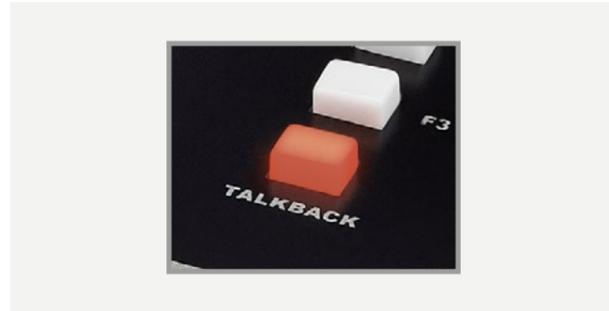
You can source the talkback audio from another audio device connected to your computer such as the built-in microphone. This allows you to free up an input channel on your iD44 that would otherwise be taken up, great for big sessions.
