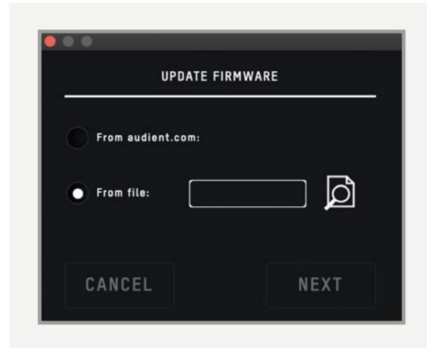
The latest version number will be retrieved from our servers and will be displayed (as shown above). Press next to continue with the firmware update. Press 'update' to install it. Once complete reboot iD44 using the power switch to apply it.
