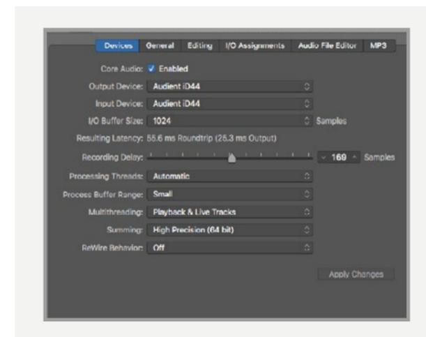
If you are using the iD mixer to monitor input signals while recording, be sure to disable Logic's software monitoring to avoid phasing as the same source will be heard twice with a short delay between the low latency DSP signal and the delayed software monitoring signal.
