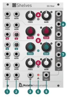
**A. High-shelf section.** This section boosts or attenuates all frequencies above the **FREQ** control. The **GAIN** potentiometer controls the amount of attenuation or boosting. No modification is applied when **GAIN** is in its central position.
